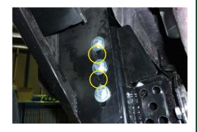
17. Mount washer bottle bracket into lefthand front corner of engine bay as shown.
