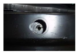
6. Open the inner holes to 12mm
