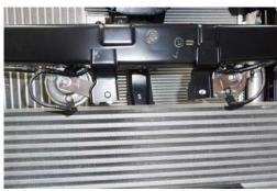
11. Unclip grill from original bumper bar at points as shown. Refit grill to vehicle using bracket supplied.
