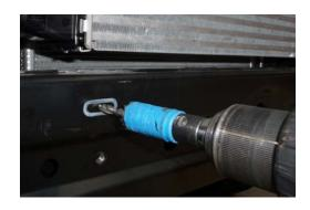
Drill a pilot hole using the centre drill bit of the hole saw through the inner skin as shown.
