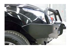
16. Once bull bar is aligned with vehicle and bolts tightened, drill through pinning holes (circled in yellow) between bull bar and chassis bracket and secure with bolts, washers and nuts provided.
