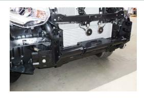
4. Mark 8 holes to be drilled through cross member and remove bull bar cradle.
