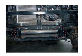
4 Trim outer bumper support brackets and mudguard liners level with bottom of radiator support panel.
