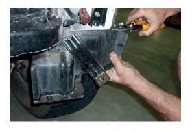
5. Fit chassis bracket to chassis using OE bolts and heavy duty flat washers supplied.
