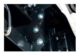
11. Fit protection plate to underneath of bull bar using M8 bolts, spring washers and flat washers provided.
