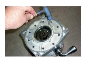
Re-install 10 bolts and tighten firmly.NOTE: Take care not to over-tighten.
