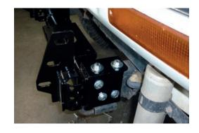
5. Refit recovery hooks using bolts supplied.
