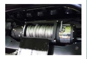
8. Bolt fairlead to recess in front of bull bar using bolts, washers and nuts provided.
