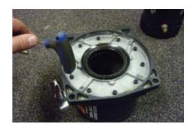
6. Refit gearbox to winch, refit and tighten Allen head bolts into tie rods.
