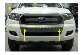
Position cutting template in place under headlight and align with guard edge and grill line.
