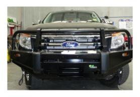
17. Fit protection plates to underneath of bull bar using M8 bolts, spring washers and flat washers provided.
