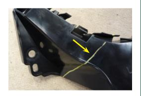
6. Mask lower edge of guard and paint lower section satin black as shown.
