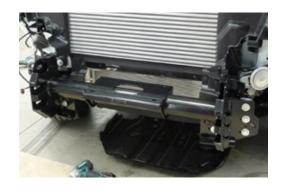
11. Using chassis bracket as a guide, drill a 12.5mm hole each side through chassis and install bolts, flatwashers, spring washers and nuts as shown.
