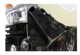
8. Remove air duct shields as shown. Disconnect temperature sensor from passenger side before removing.
