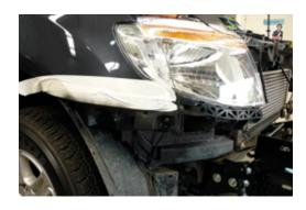
4. Measure 100mm from point on bumper bar as shown, and mask down bumper bar from this point.
