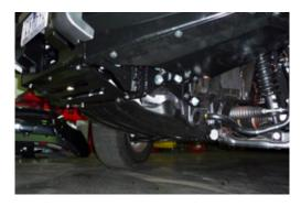
Trim guard liners using protection plates as a guide. Attach to protection plates using clips provided.
