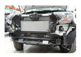
4. Temporarily re-fit top section of bumper bar (cut in previous step) to vehicle. Using end of bumper bar as a guide, mark cut lines onto plastic bumper support brackets.
