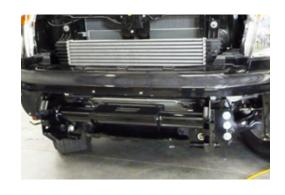
9. Using chassis bracket as a guide, drill a 12.5mm hole through chassis and install bolts, flatwashers, spring washers and nuts as shown,
