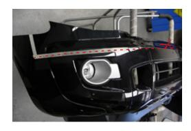
6. Temporarily refit top section of bumper bar (Cut in previous step) to vehicle. Using end of bumper bar as a guide, mark cut lines onto plastic bumper support brackets.
