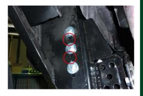
17. Fit protection plates underneath the bull bar using M8 bolts, spring washers and flat washers provided.
