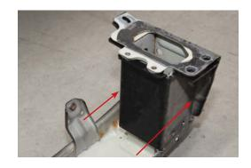
4. Drill out spot welds with 6mm drill.
