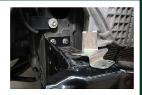
7. If winch is being installed, it needs to be attached to mounting cradle before cradle is attached to the vehicle.
