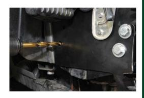
11. Open up access hole under frame as pictured to allow installation of nuts.
