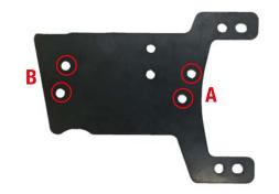
9. Fit side plates to winch cradle. Drill 10mm hole through factory bumper support bracket and support bracket as pictured. Fit supplied bolts
