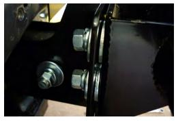
Using holes in inner and outer of chassis strengthening brackets as a guide, drill a 12.5mm hole and install a mounting bolt washer, spring washer and nut. Tighten all bolts.
