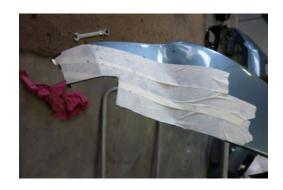
10. Cut along lines previously marked to remove sections as shown.
