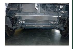
9. Remove recovery eyes and tie down points from chassis.
