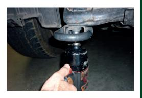
10. If your mounting cradle does not have an extra mounting hole as shown in pic A, refer to the measurements in pic B and drill a 14mm diamenter hole as shown
