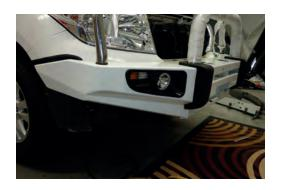
19. Once bull bar is aligned with vehicle and tightened, drill through pinning holes (circled in red) between bull bar and chassis bracket and secure with bolts, washers and nuts provided.
