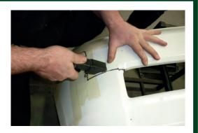
8. Remove aluminium bumper reinforcement and mounting brackets from chassis.
