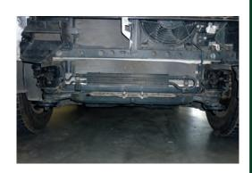
9. Remove recovery eyes and tie down points from chassis.
