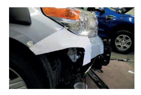
5. Mark a horizontal cut line across bumper, level with the top of the lower grill section and fog light housings as shown.
