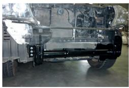
12. Insert threaded anchorplate supplied, into the rectangle shaped hole in the side of the chassis as shown in pic A.
