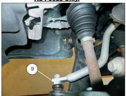
The prefered method for High spec bolt installation is to have the bolts installed from the top side of the subframe. This however requires the oval or lowering of the engine subframe and is a lengthy process. To ease installation the bolts can be installed opposed to each other or from the bottom upwards(Same as OEM). In the unlikely event that the retaining nuts may come loose and fall out it is recommended to install
